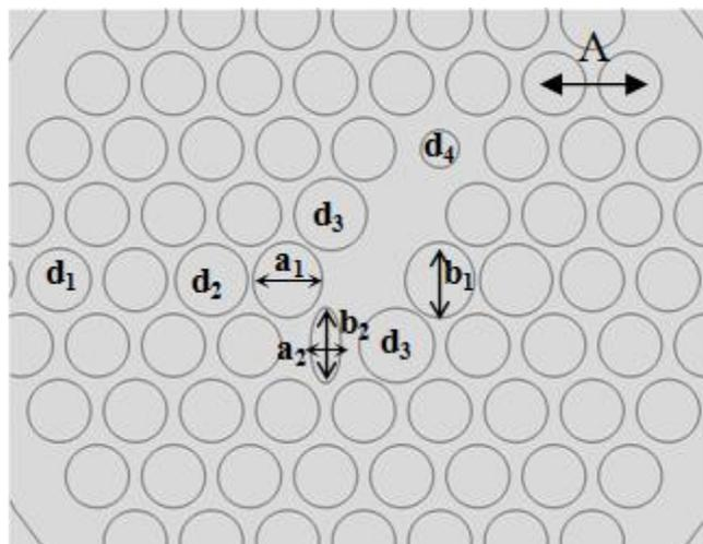
**Fig. 1** Transverse cross section of proposed H-PCF where,  $\Lambda=0.91\mu\text{m}$ ,  $d_1/\Lambda=0.83$ ,  $d_2/\Lambda=0.95$ ,  $d_3/\Lambda=0.9$ ,  $d_4/\Lambda=0.5$  and for elliptical air holes  $a_1/\Lambda=0.83$  &  $b_1/\Lambda=0.91$ ,  $a_2/\Lambda=0.36$  &  $b_2/\Lambda=0.91$ .
